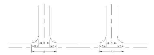
Commercial "ONE WAY" drives shall have a minimum separation of 70' center to center see rule 6.1.7 C
